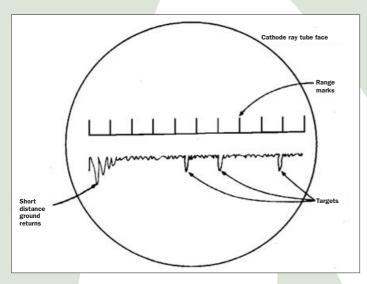
Fig. 5: A re-drawn wartime illustration showing the display presented to the operators at a CH station. The cathode ray tube (c.r.t.) was approximately 305mm (12 inches) in diameter.
