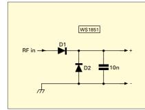
Fig. 1: This detector circuit has been used by G3RJV and uses a voltagedoubler based on the diodes, D1 and 2 (see text).
