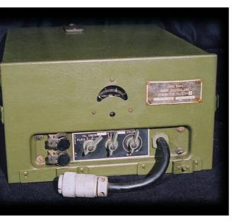
• Fig. 3: The restored BC-620 'Jeep' set. A similar sized box housed the batteries underneath (see text).
