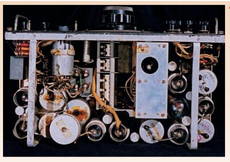
Fig. 2: The R1155 removed from its cabinet and with photograph taken from above. The 'magic eye' tuning indicator is mounted within the tubular housing on the left (wiring for the valve base can be seen), the main variable capacitor for tuning can be seen directly in line with the main tuning dial. The b.f.o. valve (valve top cap visible) in its own screened compartment to the right of the tuning capacitor. (see text).
