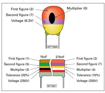
Fig. 4: Showing how colour coding is provided to show both the value, tolerance (see text) and voltage of capacitors. Note that some capacitors with colour coding can be polarised (i.e. marked + or -) and must be connected in circuit correctly (see text).
