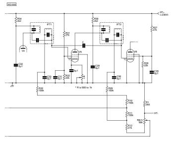
Fig. 6: Partial circuit diagram, showing the area and modifications needed to add the G3ASG 'Q-multiplier modification (see text).
