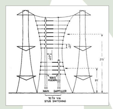
Fig. 2: Historical diagram illustrating the lay-out of the transmitting antennas at a Chain Home transmitter (see text).
