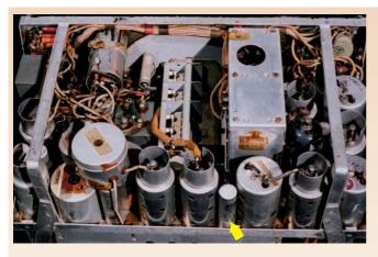
Fig. 3: Rear view of the R1155. Just to the right of the central valve (with valve top cap lead running from main tuning capacitor) is one of the multiple-capacitor-in-acan decoupling capacitors (arrowed) which feature in G3ASG's article These capacitors are notorious for becoming very 'leaky' in old age and advice is given regarding their replacement (see text).
