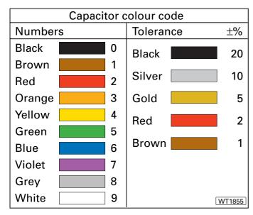
Fig. 3: Chart showing the colour code used for capacitor value marking. Please note that although it's the same as that used for resistors, important extra information is provided - please see Fig. 4 for explanations.
